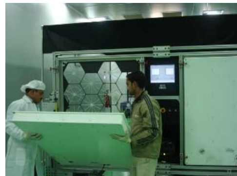
Figure 6: Loading a module into the motion frame
